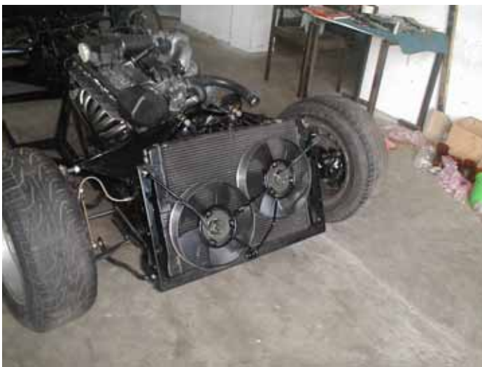
E28 535i radiator and two Toyota fans On fabricated frame and cowls
