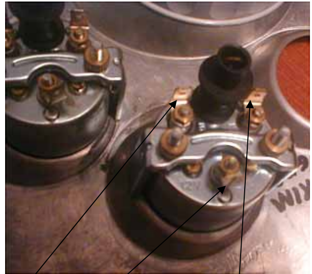
B+ Violet Brown Ground B- or T- coloured wire
